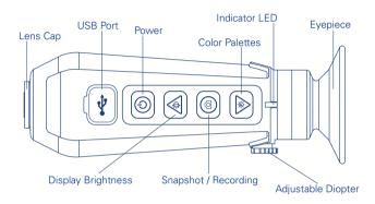
**Charging the SCOUT-TK** – Use the included USB Cable and connect to a power source. The Indicator LED flashes while charging and blinks green when fully charged.
